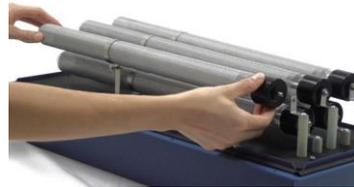
6. Secure the tube on the unit at the end cap first, using the supplied friction nut, taking care not to over-tighten. **It is important to only hold the tube by the end cap when tightening;** otherwise the outer mesh may twist, reducing effectiveness.
