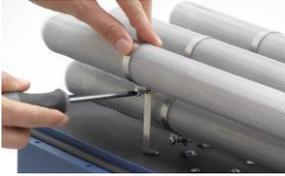
4. Loosen the screw in the end clamp around the tube. It is not always necessary to completely unclamp the tube; however, sometimes it is much easier to remove the tube by doing so.
